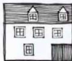
Loft conversion incorporating gabled dormers which are out of scale and do not consider existing window rhythm nor frequency.
