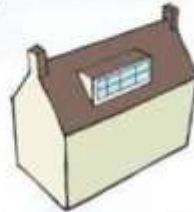
Loft conversion incorporating a long shed dormer which is out of scale with the original building.
